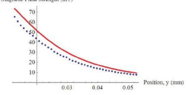
The two disk model approximation is shown in red while our experimental data is shown as blue points.
