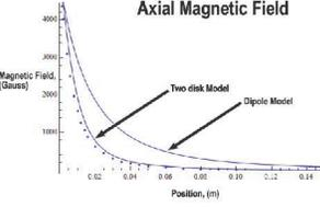
The two disk model approximation is shown in red while our experimental data is shown as blue points.
