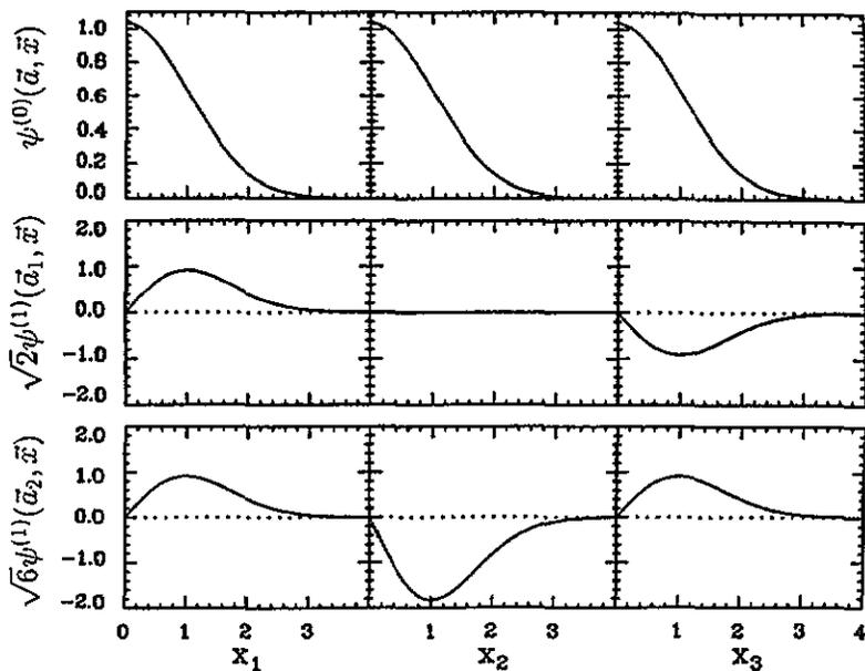
Figure 3. The three lowest eigenfunctions (equations (8)–(10)) for a three-prong harmonic oscillator potential  $V(x_i) = \frac{1}{2}m\omega^2 x_i^2$ . The ground state  $\psi^{(0)}$  is non-degenerate, whereas the first excited state  $\psi^{(1)}$  is doubly degenerate.
