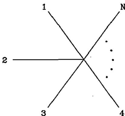
Figure 1. Schematic diagram of an  $N$ -prong potential. The position on any prong  $i$  is specified by the positive coordinate  $x_i$ , with  $x_i = 0$  being the vertex. The angles between prongs play no role in any computations.
