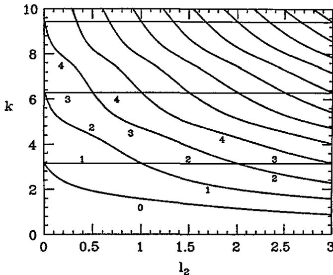
Figure 5. The eigenvalues  $k$  (energy  $E = k^2$ ) for a three-prong free particle potential as a function of  $l_2$ , the length of prong 2. The lengths of the other two prongs are kept fixed and equal  $l_1 = l_3 = 1$ . Note the pattern of degeneracy and level crossings. The curves are labelled by the number of nodes in the wavefunction (in all prongs).
