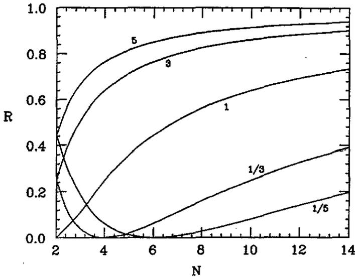
Figure 7. A plot of the reflection coefficient  $\mathcal{R}$  versus the number of prongs  $N$ . The incident wave with energy  $E$  is on prong 1 with zero potential. All other prongs are taken to be at a constant potential  $V_0$ . The curves are labelled by the parameter  $\zeta \equiv \sqrt{1 - V_0/E}$ .
